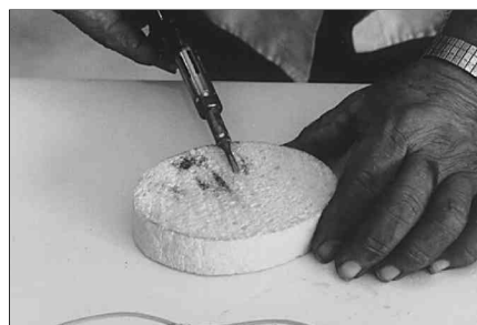
Step 5: Clean tip of soldering iron on damp sponge.
