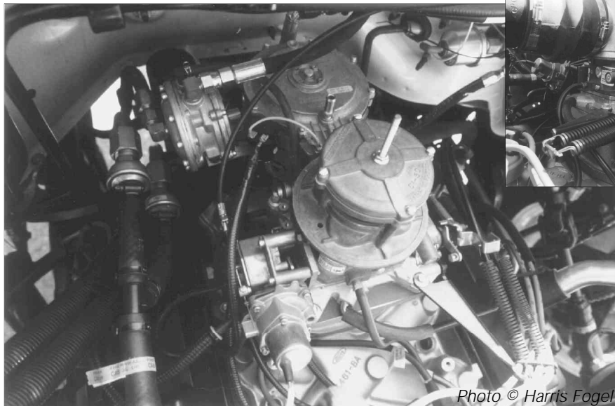
15-1 Air-fuel mixer mounted with throttle – dedicated mono-fuel application. Inset Mixer with air cleaner hood.
