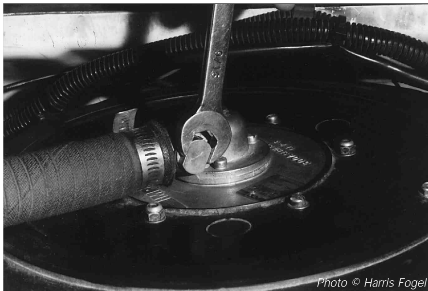
Figure 21-4 Power valve adjustment, air-valve mixer shown.
