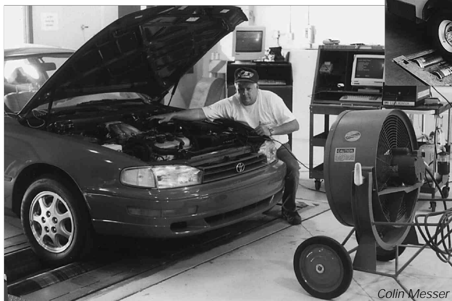
Figure 21-3, FWD vehicle positioned on dynamometer rollers, external cooling fan and test equipment in place. Inset RWD vehicle on rollers.
