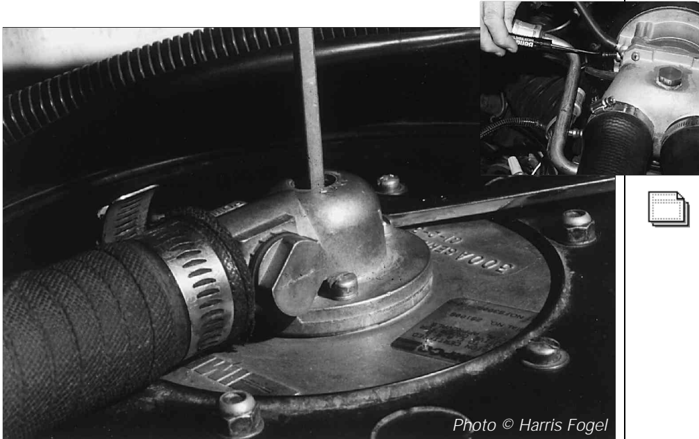
21-5 Idle air-fuel mixture adjustment.
