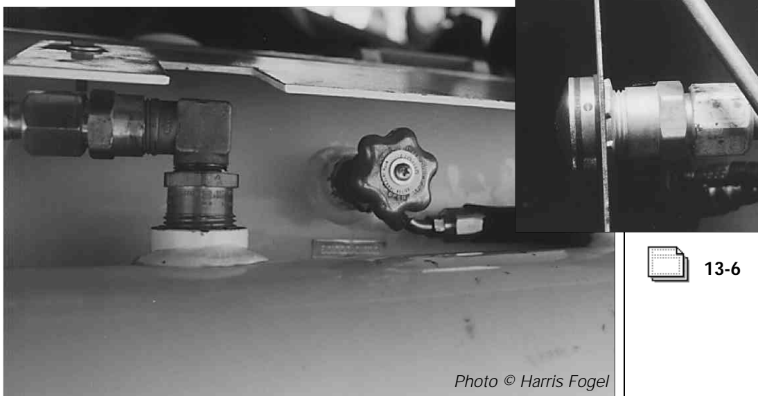
13-3 Relief valve remote pipe-away. Inset Rain/dust cap for relief valve pipe-away.
