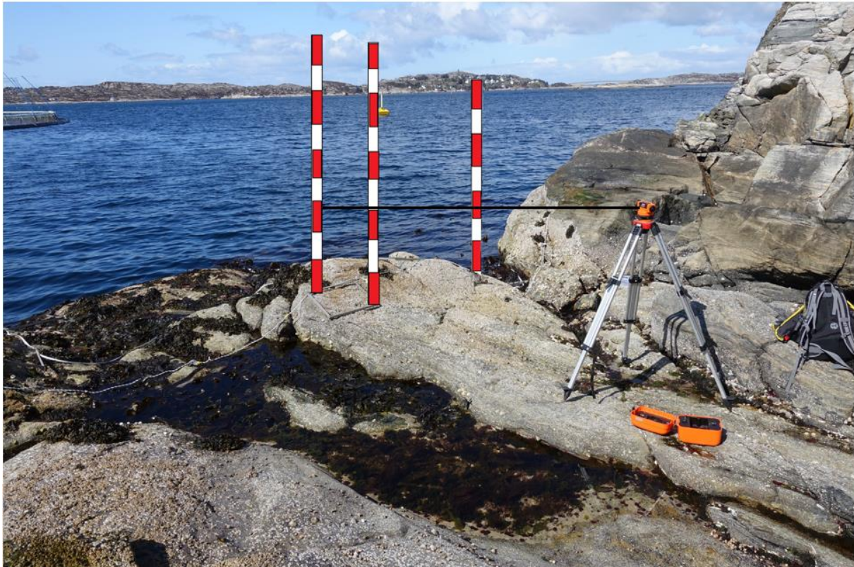
Figure 5 – Figure showing monocular and how the vertical height was measured. The measuring rod to the left is measuring the highest point on the quadrant, the one in the middle the lowest point, and the one to the right is measuring the water level. The black line indicates the view through the monocular.
