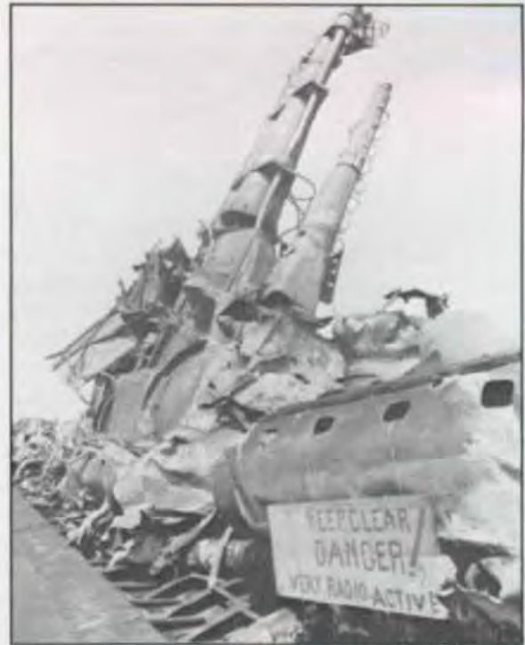
USS Skate in the aftermath of Able , its superstructure crushed, conning tower bent, and "very radio-active." (National Archives)
