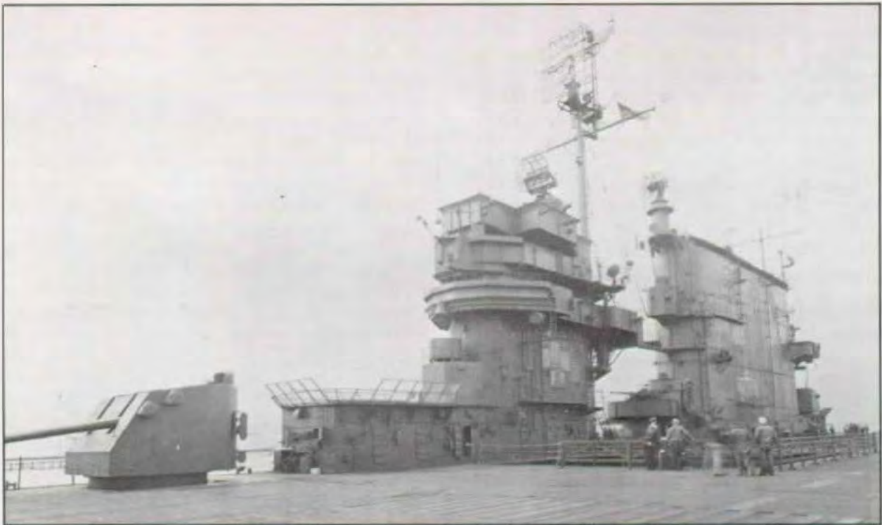
Saratoga's island, stack, and No. 1, 5-inch mount after stripping the ship for Crossroads. This photograph was taken at the Naval Air Station, Alameda, California, February 27, 1946. (Flouting Drydock)
