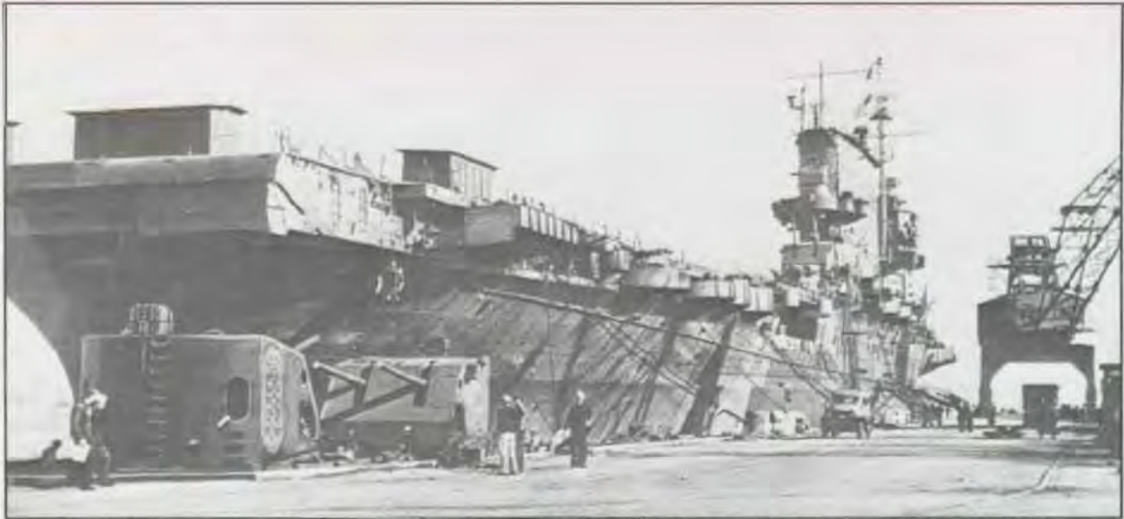
Saratoga being prepared for Operation Crossroads at Hunter's Point. Note the two 5-inch/38 caliber gun houses landed on the dock off the carrier's stern. (San Francisco Maritime National Historical Park)
