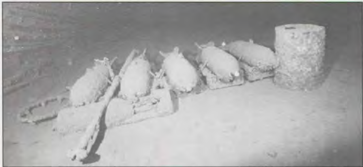
Five general purpose 500-lb. bombs, AN-Mk 64, on their bomb carts, on the starboard side of Saratoga's hangar deck at frame 82. Lying forward of the bombs is a single 350-lb. depth bomb, AN-Mk 64, originally stowed with four others on the port side, which rolled free and lodged against the 500-lb. bombs. (National Geographic Society, Bill Cutsinger)
