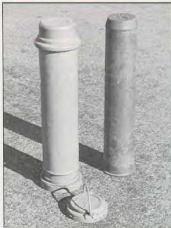
Five-inch cartridge case, showing the cartridge. The warhead was added by the gun crew in the handling room. (NPS, Canduce Clifford)
