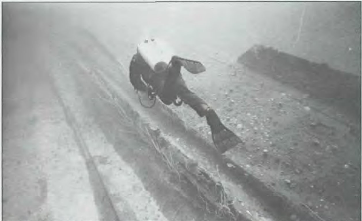
Daniel Lenihan swims forward past the port bilge keel of Arkansas . Longitudinal failure of the shell plating resulted in the long dents in the hull. (NPS, Larry Murphy)
