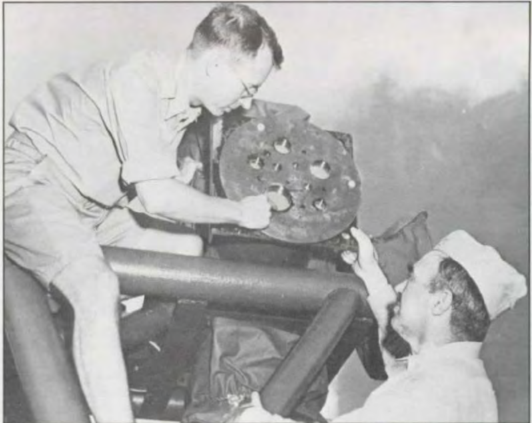
Installing a ruptured foil peak pressure gauge on a "Christmas Tree," in 1946. (U.S. Naval Institute)
