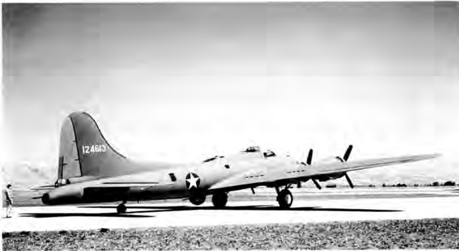
The Boeing XB-17F with turbocharged engines (1942).
