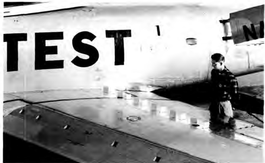
Vortex generators mounted on the wing of a North American YF-86D.
