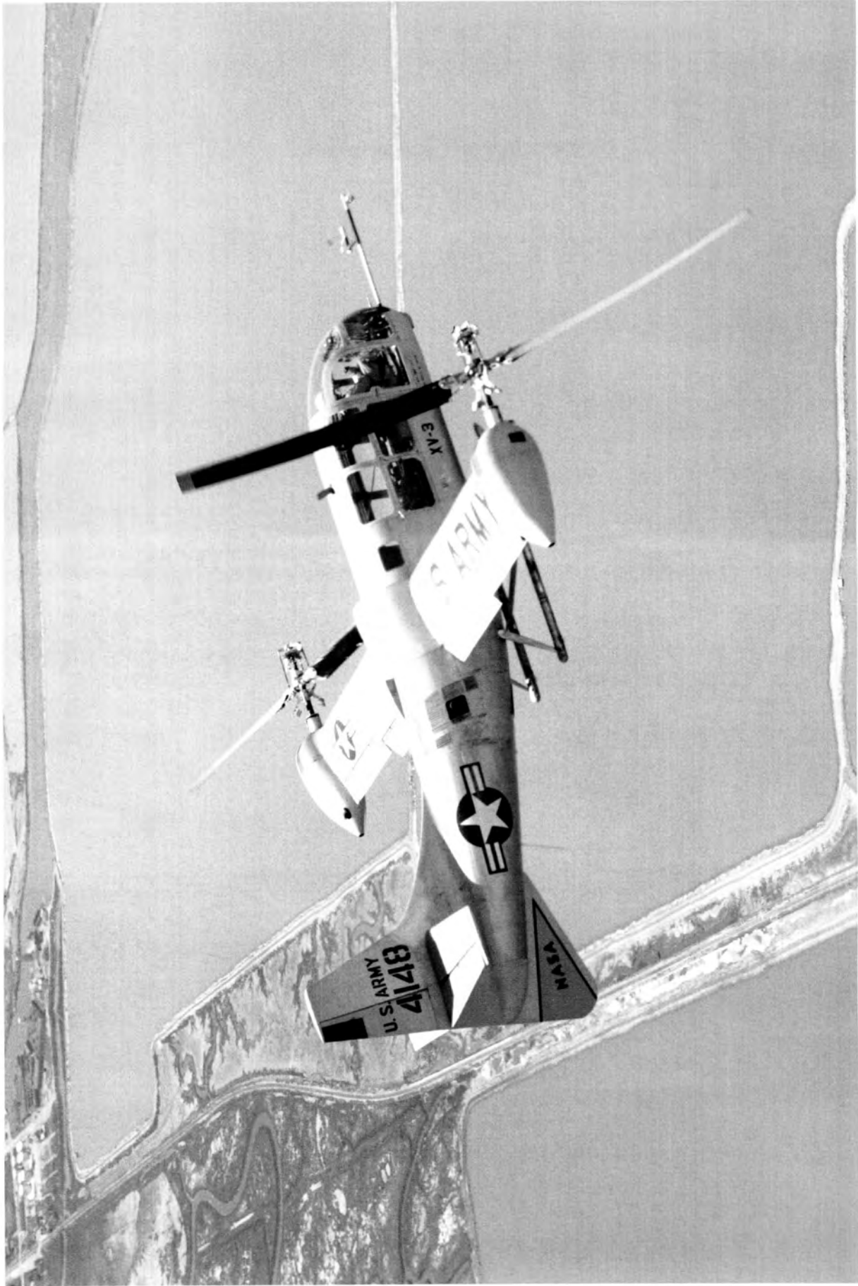
Figure 86. Bell XV-3 with rotors fully tilted for conventional cruise flight. Note large rotor-blade angle which reduced pitch and yaw static stability. Maximum cruise speed of the XV-3 was limited to 140 knots because of low damped lateral-directional oscillations. (Apr. 1961) A-26672
