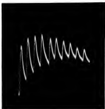
FIG. 3.—Electric response of metal showing fatigue (tin).
