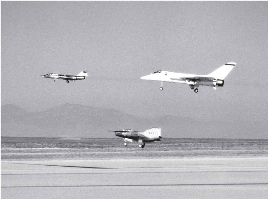
Observers in chase planes, including the F-104 (left) and the F5D-1, kept a close eye on the M2-F2 during each flight. (NASA)
