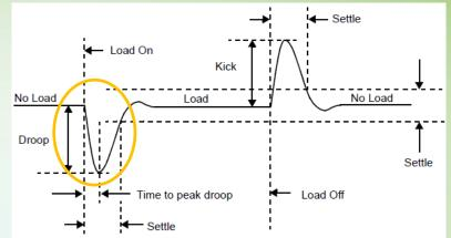
Time domain response of the Power Supply to transistor switching Large droop → Yield below targets and/or lower device specs
