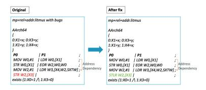
Litmus test results (executed 50000000 times on a certain Arm server) are shown below. The test results of original code contain some (X0=1; X3=0) cases (51 times in all the 50000000 test), which violate the essential program logic. No such (X0=1; X3=0) violation cases are found for the fixed code.
