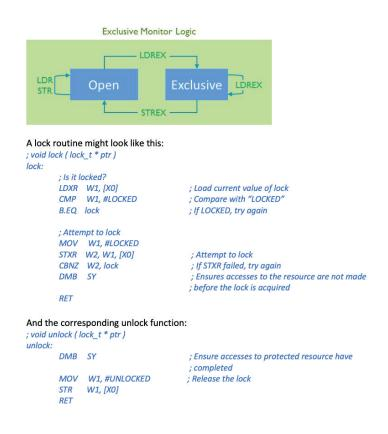
Note that STXR is not required in an unlock operation. It is only used when testing and setting it in a lock operation.
