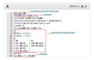
In the mp.litmus test, the "PodWW Rfe PodRR Fre" is the examined sequence of candidate relaxation (memory operation relation). Then, the assembly code is generated corresponding to the specific candidate relaxations. The last "exists" statement is the final state to be checked whether existing.
